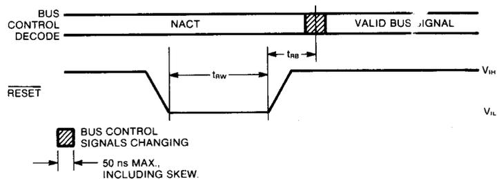
**Fig. 38 LATCH ADDRESS TIMING**
