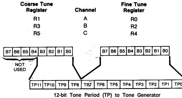
Note that the 12-bit value programmed in the combined Coarse and Fine Tune registers is a period value—the higher the value in the registers, the lower the resultant tone-frequency.
