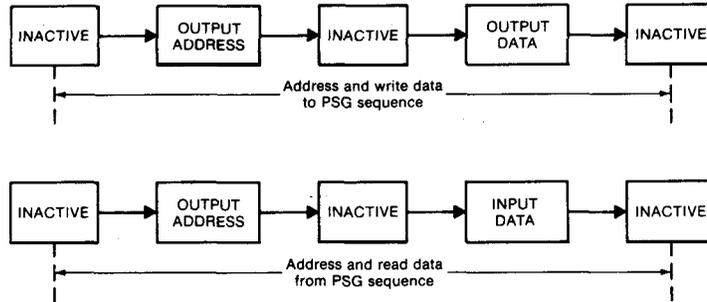
The functional operation and relative timing of the PSG control sequences are described in the following paragraphs (in all examples, BC2 has been assumed to be tied to logic "1", +5V).
