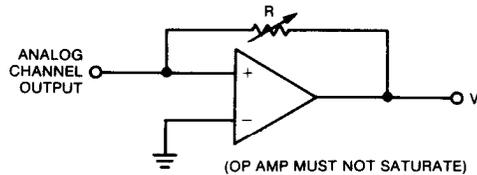
Fig. 35 CURRENT TO VOLTAGE CONVERTER
